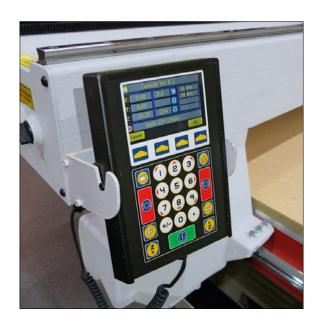
The AXYZ SmartConsole brings unprecedented ease of use, context sensitive menus, real-time display of machine status in addition to many more time-saving, functional and productivity features. It provides a graphical preview and current status of a running job and allows program feeds and speeds to be changed without pausing the program.
