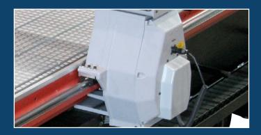
The steel gantry runs on high-quality linear bearings and is driven on both sides by servo motors coupled through planetary gearboxes. This provides a strong transmission for quality high-speed machining and auto-squaring of the gantry for precise alignment at all times.
