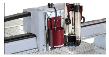
The versatility of the oscillating and tangential knife cutting units allow processing of an expansive range of materials with ease and precision. Combine a routing spindle with an automatic tool-change and add one or more knife tools for maximum flexibility to process a massive range of rigid and semi-rigid sheet materials.
