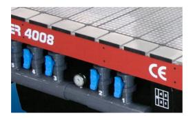
The vacuum deck can be configured with either standard vacuum zones or they can be customized for specific requirements and part sizes.
