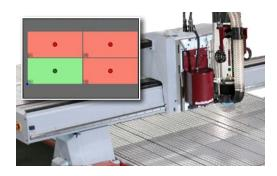
Auto-zone management allows the router to operate in Live Deck mode which will automatically activate and deactivate zones according to the live position of the cutting head.
