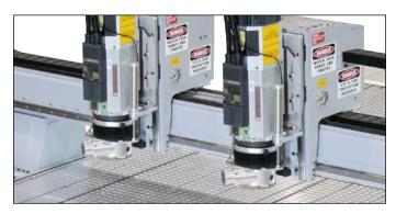
The twin-carriage option allows two parts to be cut simultaneously, effectively doubling production capacity and enabling faster job turnaround.
