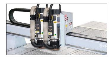
Choose a single, double or even triple-head carriage for multiple tasking operations that typically require only two or three tooling processes. Rout, profile, trim and drill in a seamless sequence. HSD router spindles feature a simple and powerful quick-release tool-change system. The manual tool-change Elte spindles provide a conventional collet and covernut alternative.
