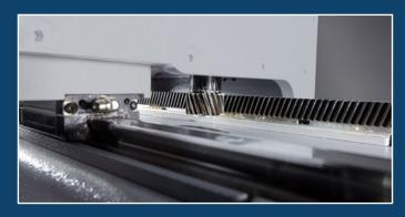
Pacer Series CNC routers achieve high-accuracy motion and cutting performance through their helical rack drive systems and high-tolerance components. They are ideal for aluminum fabrication, aerospace component manufacturing, plastic fabrication and many other demanding situations.
