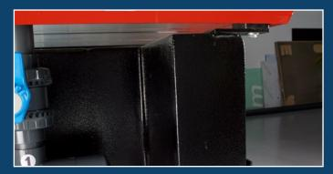
All Pacer series machines are built on a heavy duty steel base which is a single piece welded and stress relieved component. This provides the perfect platform for high speed, vibration free processing of even the toughest materials.
