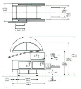
Mechanically the T-350 trim press is similar to the T-300 model but offers a wider platen opening to accommodate sheet widths up to 52". Its capacity is rated at 30 tons for trimming small, medium, or large plastic parts produced by the Brown C-4600 Series Continuous Thermoformers.
