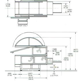
Rated at 30 tons, the Brown T-300 trim press is designed to trim small to medium sized parts in thicker and tougher materials. It is ideally suited to work in-line with Brown Machine's C-4200 sized thermoforming machines, or other machines of similar capacity.
